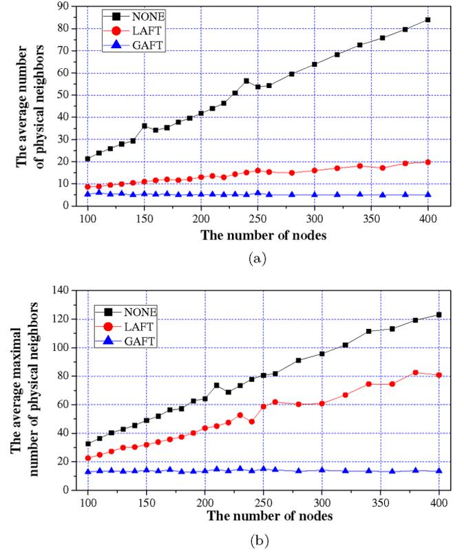
**Figure 7** Comparison of GAFT and LAFT with respect to the ratio of LD to PD, where LD and PD refer to degree and the number of physical neighbours (see online version for colours)
